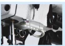
The humanized LED lamp make the operator place fabrics more accurately and reduce the eye fatigue of operators.
