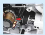
The Up and down shaft is transmitted by timing belt, so the noise is low and the machine is more lightly.
