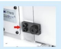
Optimized design for mechanism of timing belt tension wheel make the tension regulation of timing belt very easy without remove the electric box and other parts.
