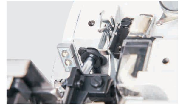
3 Fully enclosed needle bar oil return device, clean sewing
